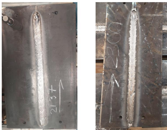
Fig. 2. Surface appearance. Left, butt welding, without filler. Right, butt welding with Ni foil.
