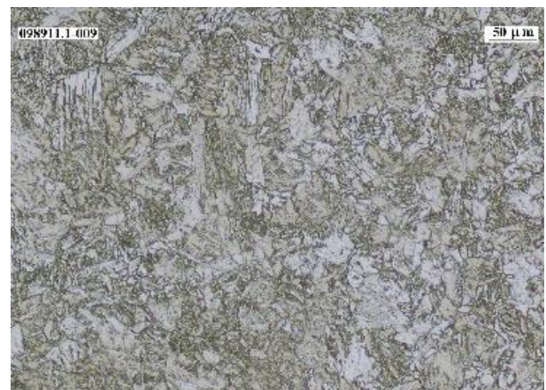
Fig. 4. Microstructure of the HAZ at mid-depth
