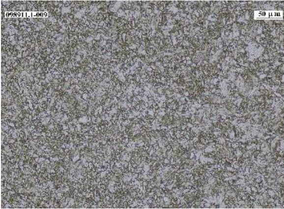
Fig. 5. Microstructure of the HAZ in the lower region.
