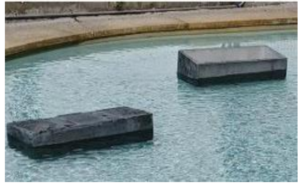
Fig.3. Small prototypes performed in preliminary trials to check production process and buoyancy.
