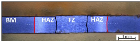
Fig. 5. Microhardness measurement macrophoto.
