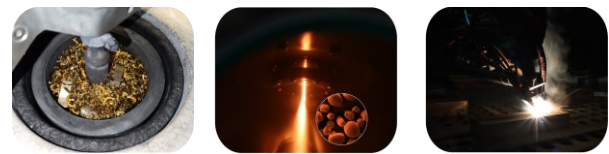
Fig. 7. Crucible with bronze shavings (left) powder atomization (middle) DED-LP process (right)
