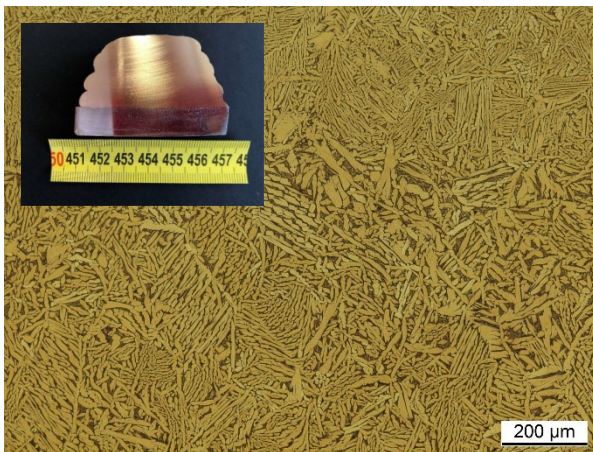
Fig. 1. Microsection of sample “163 A | 20,2 V” with primary \alpha -phase
